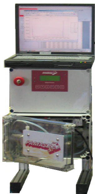
FIGURE 1 PHOTO OF THE PAMAS WATERVIEWER PARTICLE COUNTER
